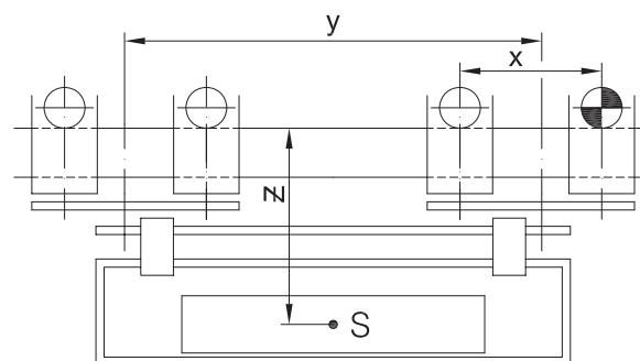
**Principle "2/4": Four running wheels / two driven wheels**
