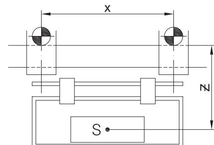
**Principle "1/4": Four running wheels / one driven wheel**
