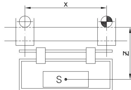
**Principle "2/2":** Two running wheels / two driven wheels
