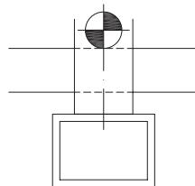
**Principle "1/2":** Two running wheels / one driven wheel
