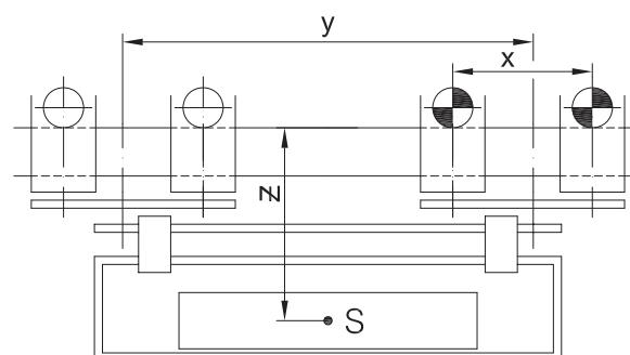
Note, "Principle 2/2" and "Principle 2/4" both involve carriages with two drives. Particular attention must be paid to cornering in such cases since different speeds will be present on the two drives when entering and exiting the corner; in practice this is resolved by the different motor slip on the two drives. This can cause considerable additional loading on the gear unit and motor, particularly where curves are tight and there are large distances between the drives wheels.
